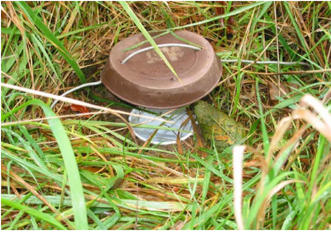
Fig. 25. Plastic cup pitfall trap in situ . Here, protection from rain is provided by a plastic plant pot saucer supported on a wire loop. © P. Smithers.
